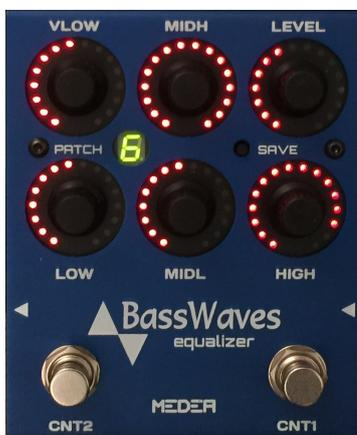
All the parameters can be adjusted using the control knobs; the equalizer frequencies are calculated for a bass guitar.
